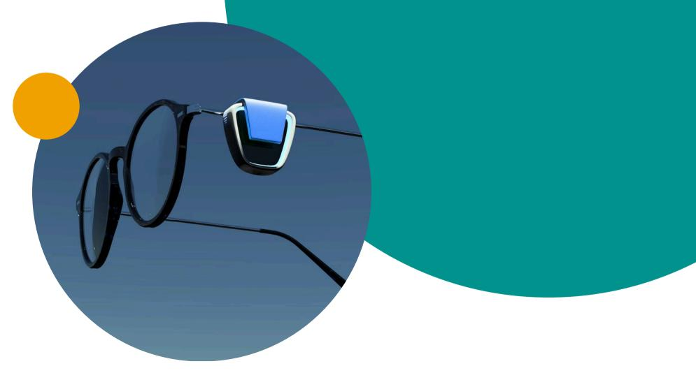
Alert Drive is a compact, smart wearable device that attaches to any glasses handle to monitor driver alertness. Using advanced sensors and microprocessors, it detects early signs of fatigue such as blinking patterns, head movement, and skin conductivity, helping prevent drowsy driving and enhance road safety.
